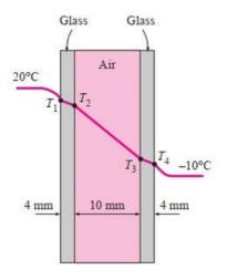
Fig. 2: Schematics of the double pane window
