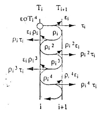
Figure 5.2 - Radiative Transfer between Adjacent Layers.
