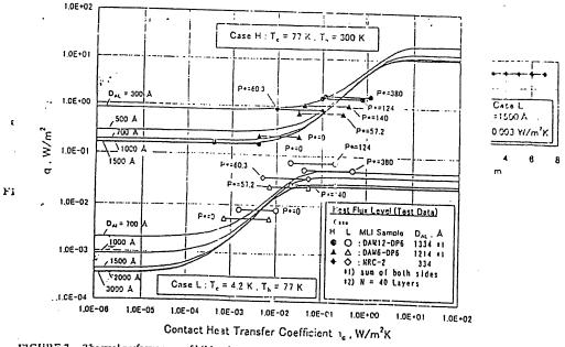
TTC FIGURE 7. Thermal performance q of MLI and contact heat transfer coefficient he between adjacent layers
