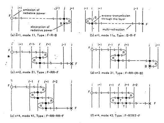
Figure 5.5. Radiative Heat Transfer from i th Layer to i + k th layer (n>0)
