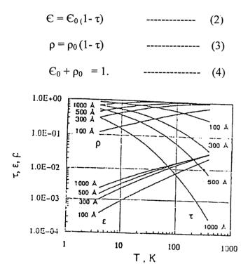
Figure 5.1 – Radiative Coefficients of Aluminum Thin Films.
