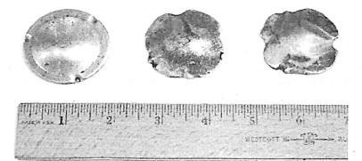
Figure 7: Cage Tray Caps after Six Month in Prefractionator Column Processing NAs Crude [42]
