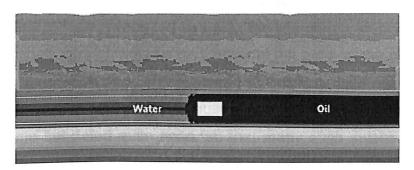
Fig.2 Dewatering of oil pipeline
