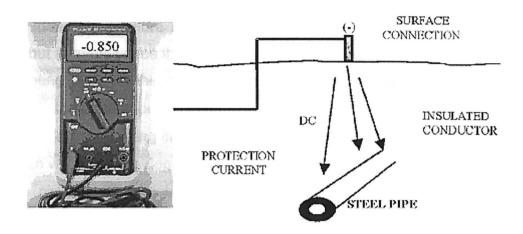
Fig.9 Criterion 1 for cathodic protection
