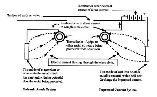
Fig. 8 Galvanic Anode System
