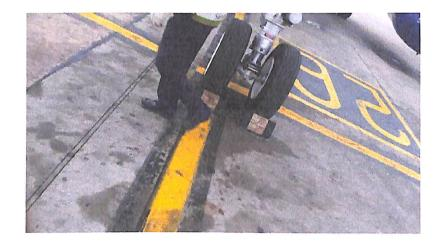
Figure 1: placing the chocks.
