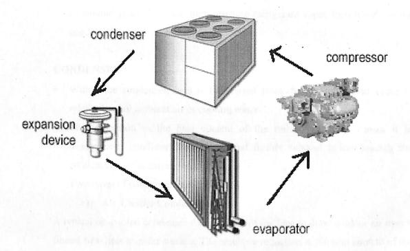
Figure7: Major component in Vapor-Compression Cycle
