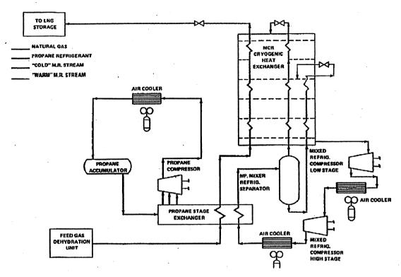
Figure 9: Liquefaction of Natural Gas Air Products Propane Precooled Mixed Refrigerant
