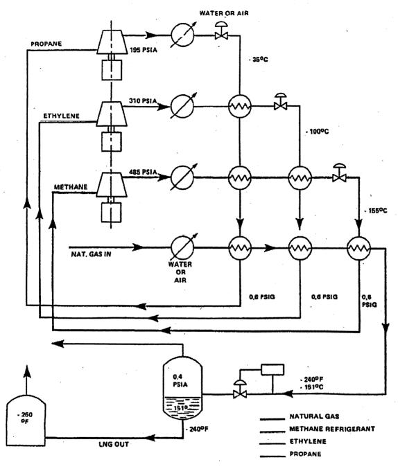
Figure 8: Liquefaction of Natural Gas Classical Cascade
