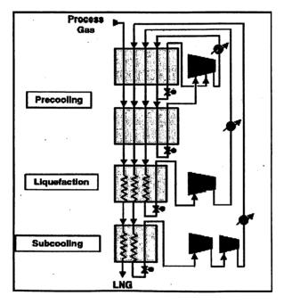
Figure 12: Linde Mixed Fluid Cascade Process
