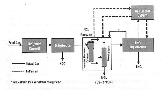
Figure 18: Block Diagram showing integrated NGL and LNG process
