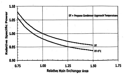
**Figure 19:** Effect of main exchanger area and propane condenser approach Temperature on specific power for a typical LNG liquefaction process
