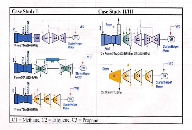
Unlike the split-shaft gas turbines, single-shaft turbines such as the Frame 7EA series turbines require starting assistance beyond what is typically provided by the vendor. For the driver/compressor configurations presented it was necessary to equip the Frame 7EA
