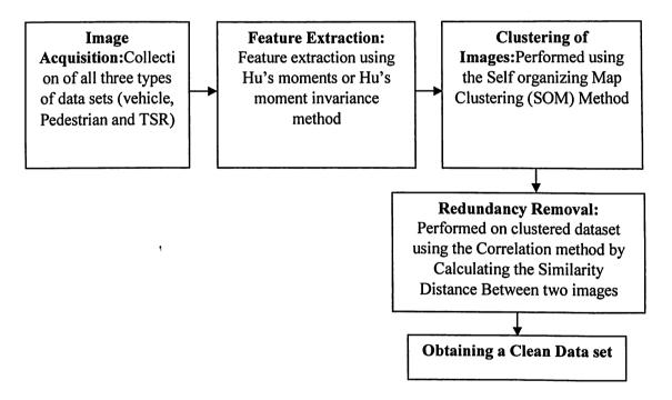
Fig. 3.5. The Basic Block Diagram of the Proposed System
