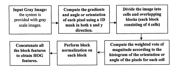
Fig. 3.6. The Basic Block Diagram of the Hog Feature Extraction Method
