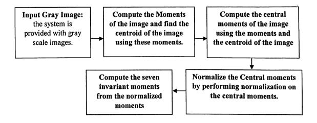
Fig. 3.7 The Basic Block Diagram of the Moment Invariant Feature Extraction Method
