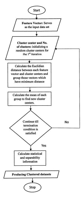
Fig. 3.4 Flowchart of the K-means Clustering Algorithm
