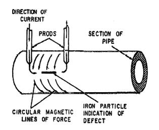
Fig.-26: Circular Magnetization (PROD Method)
