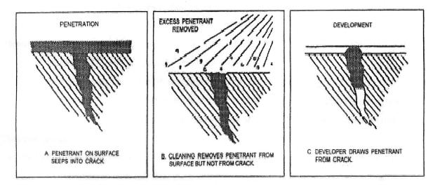
**Fig.-28: Liquid Penetrant Inspection**
