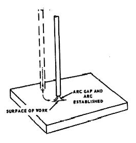
Fig.-8: Tapping method of starting the arc
