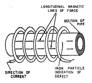
Fig.-27: Longitudinal Magnetization (COIL Method)
