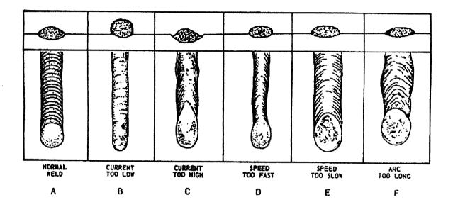
Fig.-9: Comparison of welds
