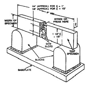
Fig.-21: Nick-Break Test of a Butt Weld
