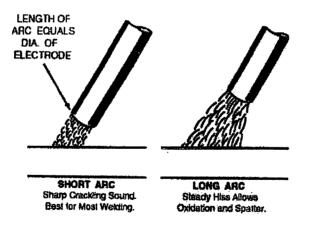
Fig.-11: Setting the length of an arc
