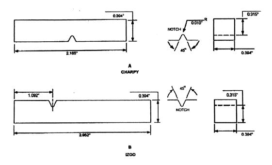
Fig.-22: Test Pieces for Impact Testing
