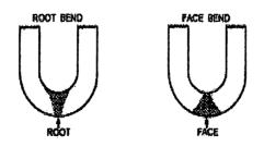
Fig.-19: Guided-Bend Test Specimens
