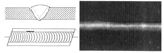
Fig.-37: External or Crown Undercut
