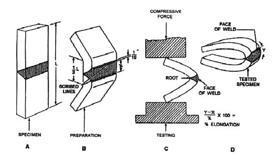
Fig.-18: Face-Bend Test
