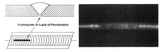
**Fig.-33: Incomplete Penetration**
