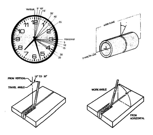
**Fig.-12: Electrode Positioning Angles**
