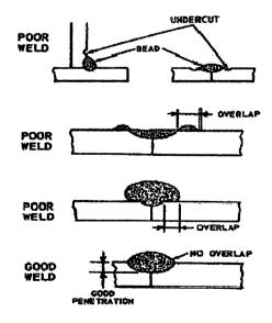
Fig.-10: Undercuts and overlaps in welding
