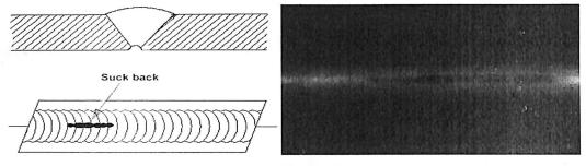
Fig.-35: Internal Concavity or Suck Back
