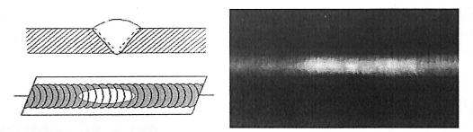
**Fig.-40: Excess Weld Reinforcement**
