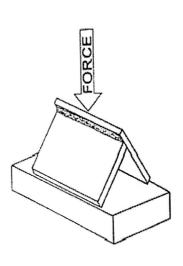
Fig.-24: Rupturing Fillet Weld Test Plate
