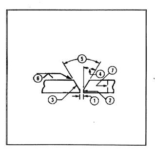
**Fig.-3: Butt Joint**
