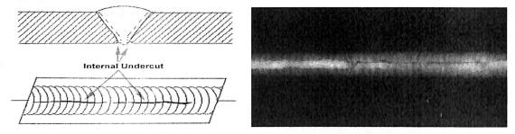
Fig.-36: Internal or Root Undercut
