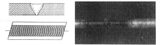
Fig.-39: Inadequate Weld Reinforcement
