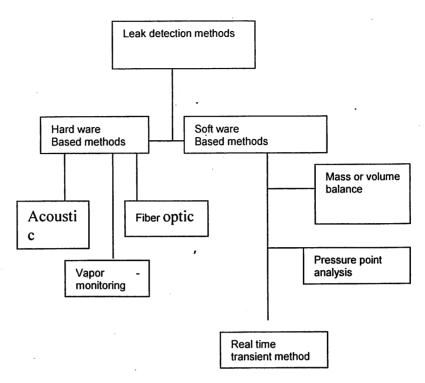
Fig 3 CATEGORIZATION OF LEAK DETECTION TECHNOLOGY
