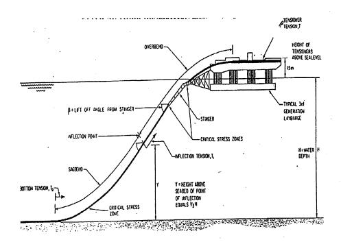
SOURCE AN INTRODUCTORY COURSE IN MARINE PIPELINE ENGINEERING BY EIL, INDIA FIG2 S-LAY METHOD
