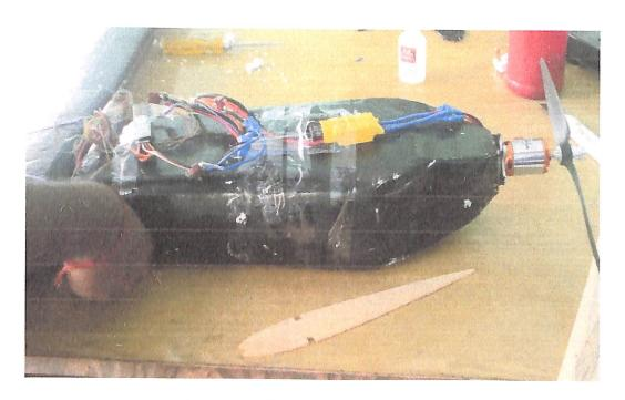
Figure 4.15: Controller assembly of UAV
