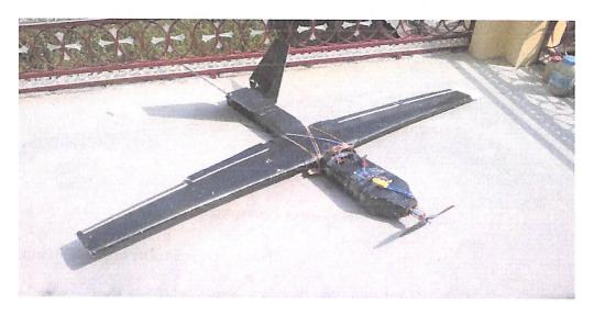
Figure 6.1: Prototype scaled model of UAV
