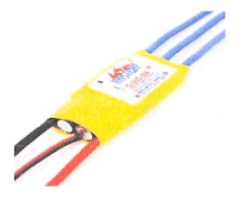
Figure 4.22: Electronic speed controller
