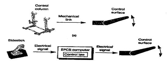
Figure 5.2: Mechanical and Electrical control
