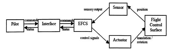
Figure 5.1: System top-level functions of the Flight Control System
