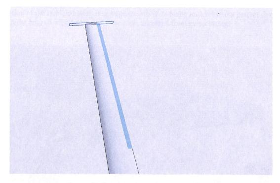
Figure 4.12: Extrude cut feature for attaching Ailerons
