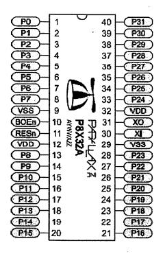
Figure 4.20: Parallax Microcontroller P8X32A-D40 40-pin DIP
