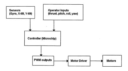
Figure 5.3: Control system schematic
