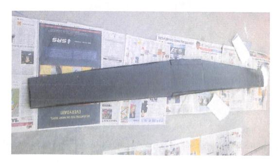
Figure 4.13: Fabrication of the wing
