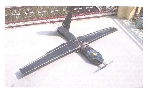
Figure 4.16: Complete prototype model of UAV
