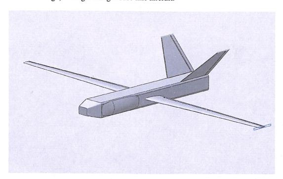
Figure 6.3: Solid work model of fabricated UAV
