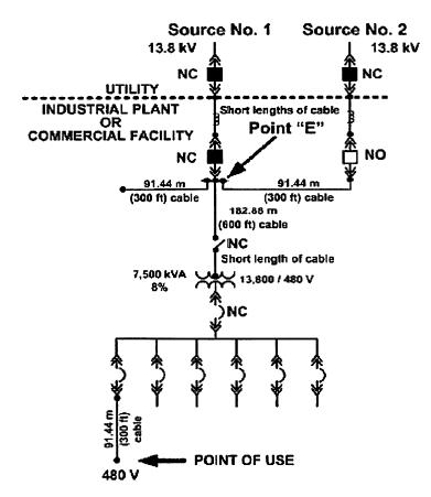
Figure-4.5-Primary-selective system to the load side of 13.8 kV circuit breaker (Example-3)
