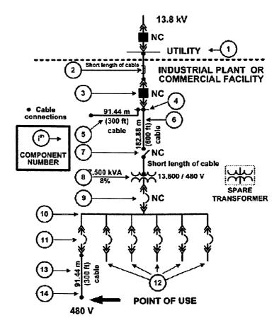
Figure-4.8 - Simple radial system with spare (Example-6)
