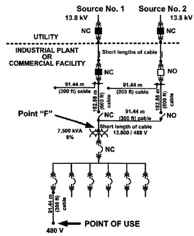
Figure-4.6 - Primary-selective system to primary of transformer (Example-4)
