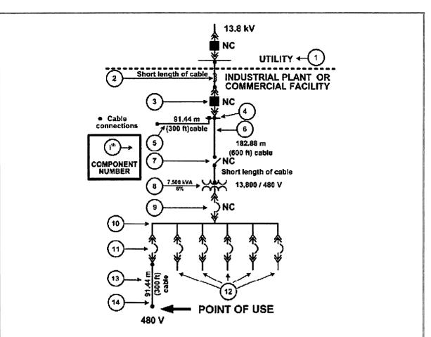
Figure-4.3- Simple radial system (Example-1)
