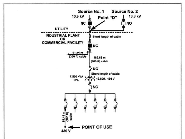
Figure-4.4- Primary-selective system to 13.8 kV utility supply (Example2)
