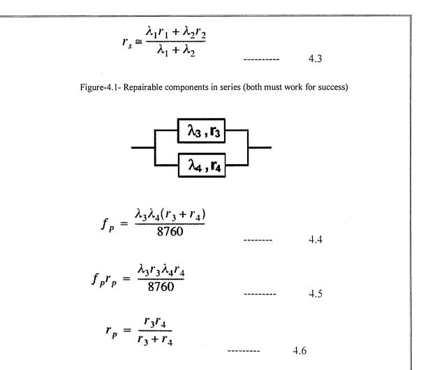
Figure-4.2- Repairable components in parallel (One or both must work for success)
