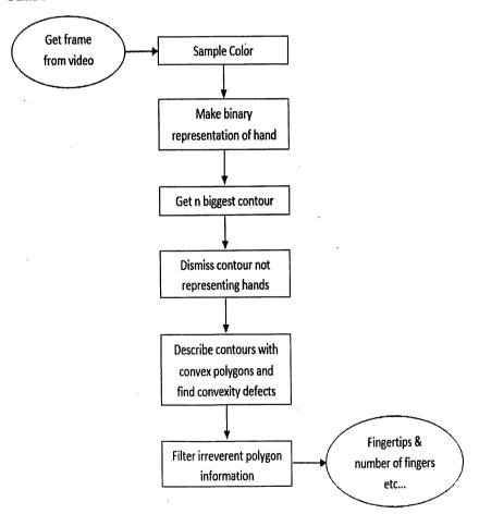
Figure 5-1 Flow chart for hand gesture recognition
