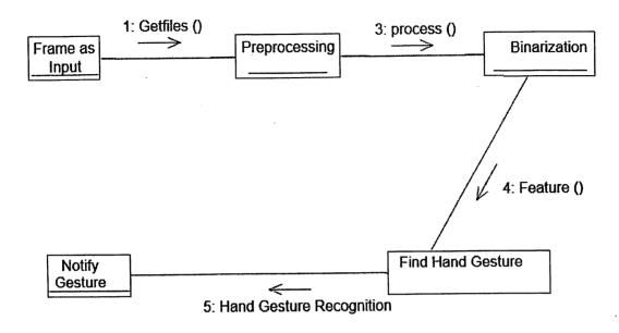
Figure 5-8 Collaboration Diagram for the proposed system
