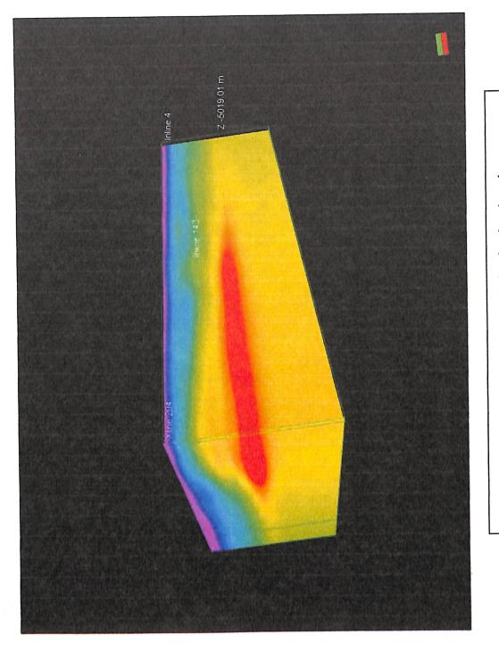
Plate 10: Final interval velocity model for depth migration
