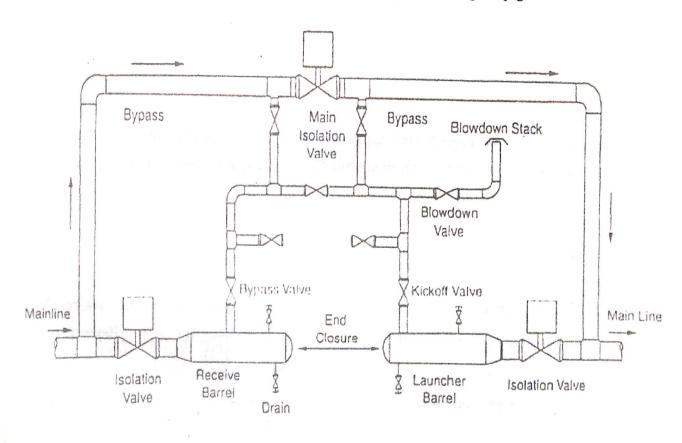
Figure 4.9: Scraper launcher/ Receiver
