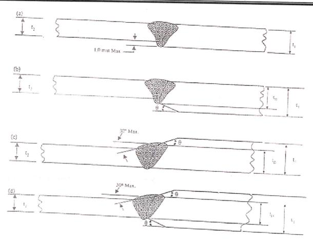
Figure 4.6:Back beveled joint design for piping design to operate at a hoop stress of 60% SMYS or less
