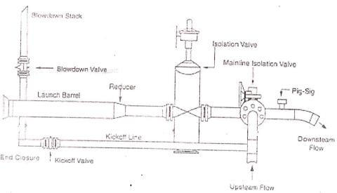
Figure 4- 12 : Typical gas line launching trap
