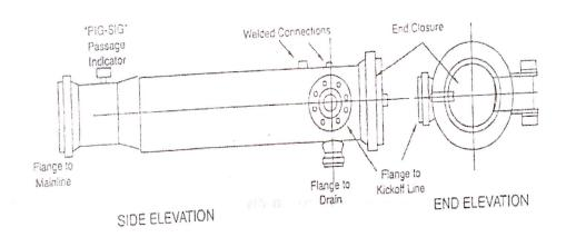
Figure 4.10:Typical Pig Launcher
