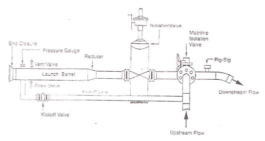
Figure 4-13: Typical Liquid line launching trap
