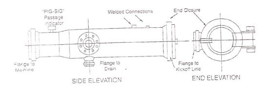
Figure 4-11: typical pig receiver
