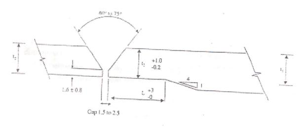
Figure 4.7 Counterbore and taper joint design for transition welds joining pipe of unequal wall thickness. Tolerances in mm.
