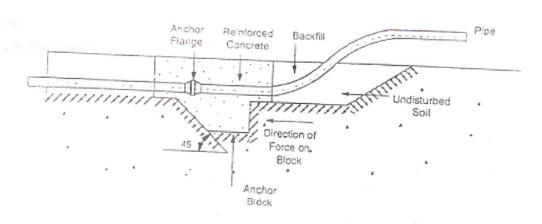
Figure 4.5 Cross-section through anchor block
