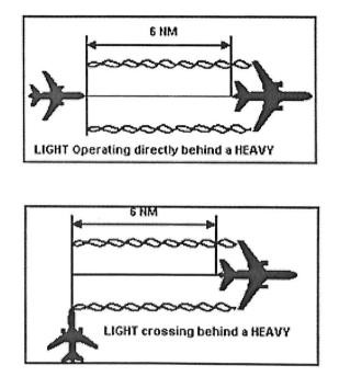
Figure 3: Separation minima based on ATS surveillance systems
