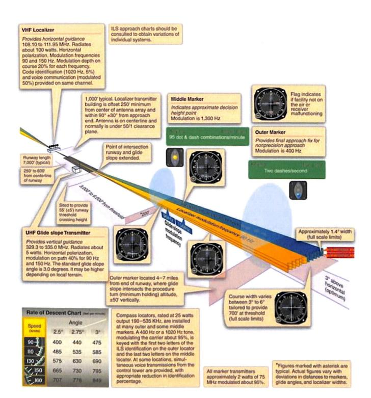
Figure 38: Instrument landing system
