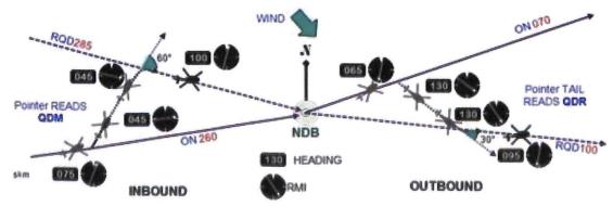
Figure 20: Intercepting the radial using RMI
