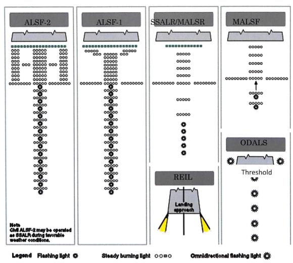
ALSF: - Approach light system with sequenced flashing lights
