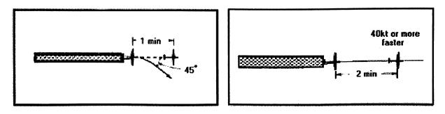
Figure 9a: Minimum separation between departing aircraft
