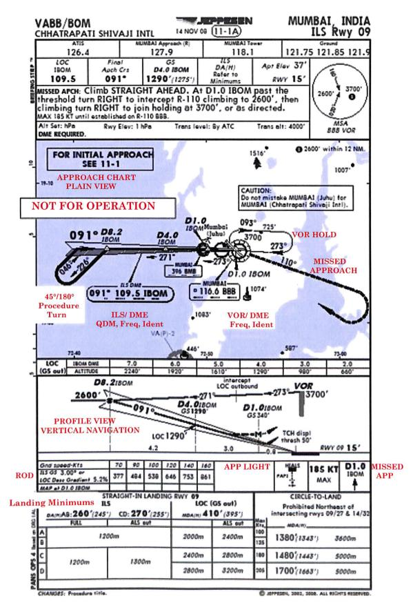
Figure 48: ILS Approach plate - Plan view/Profile view
