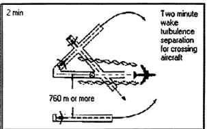
Figure 13: Wake turbulence minima for departing aircraft
