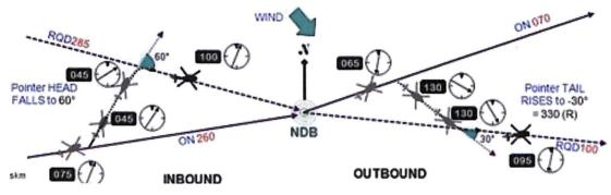
Figure 19: Intercepting the radial using ADF Indicator
