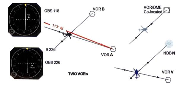
Figure 27: Using two NAV AIDS to fix position
