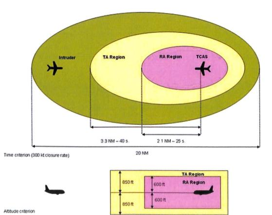
Figure 52: Example of a typical TCAS protection volume
