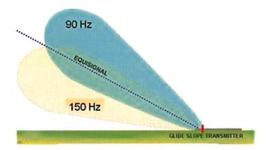
Figure 40: Glide Slope radiation- Plan view
