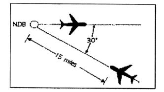
Figure 6b: Lateral Separation using NDB
