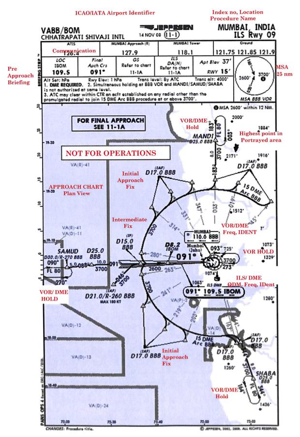
Figure 47: ILS Approach plate - Plan view
