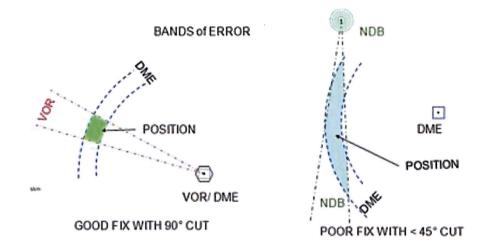
Figure 36: Fixing position with DME
