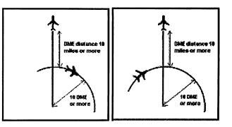
Figure 10: Departing aircraft is maintaining a radial from a VOR and arriving aircraft established on a DME arc
