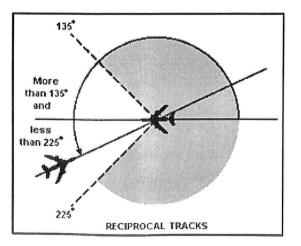
Figure 7b: Longitudinal separation Reciprocal tracks
