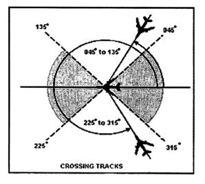
Figure 7c: Longitudinal separation crossing tracks
