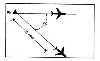
Figure 6c: Lateral Separation using dead reckoning
