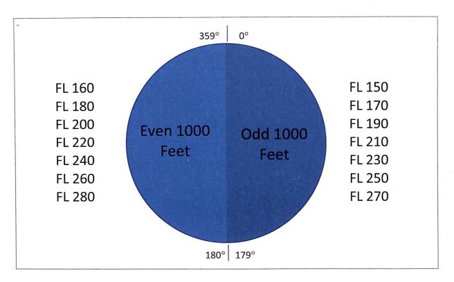
Figure 5: Semicircular system for vertical separation
