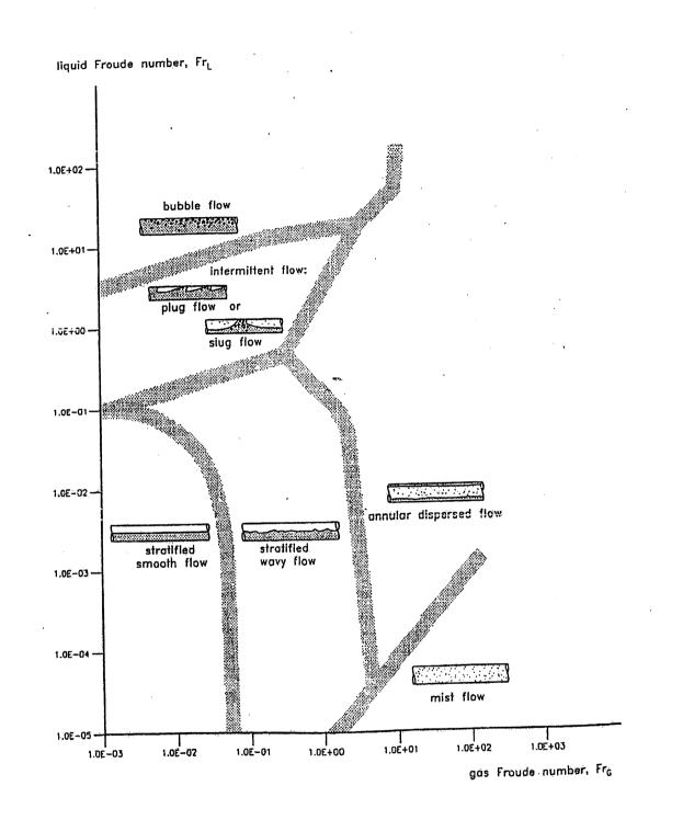
Fig 8.5 Two phase flow maps for Horizontal feed pipes
