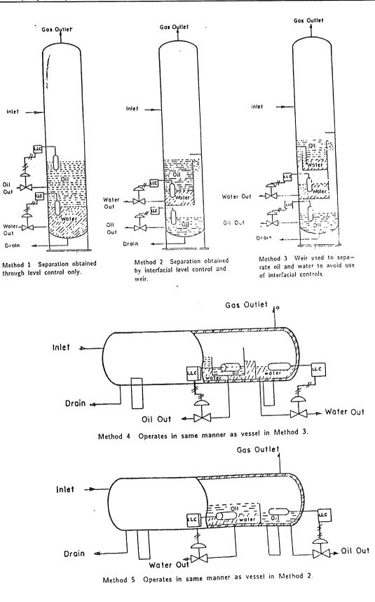
Fig.6.3 Various methods for controlling Three-phase Separation
