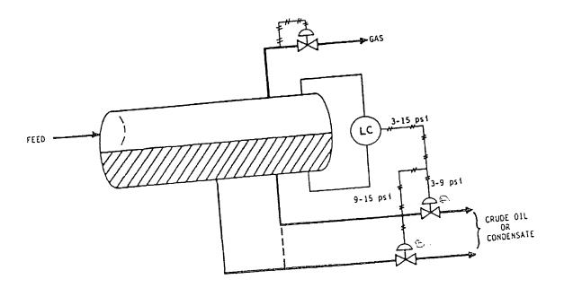
Fig.6.1 Example of a split-Range level control
