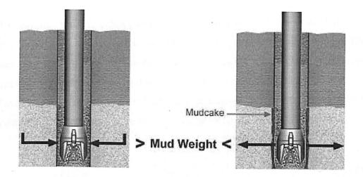
Besides minimizing lost circulation and increasing the penetration rate, this technique has a widely recognized benefit of minimizing the damage caused by invasion of drilling fluid into the formation. In many UBD applications, additional benefits are seen due to reduction in drilling time, increased bit life, and early detection and dynamic testing of productive intervals while drilling. It is critical to keep the well underbalanced at all times, if formation damage is to be minimized.
