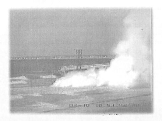
Fig-18 Physical explosion: LNG RPT Source: Internet image
