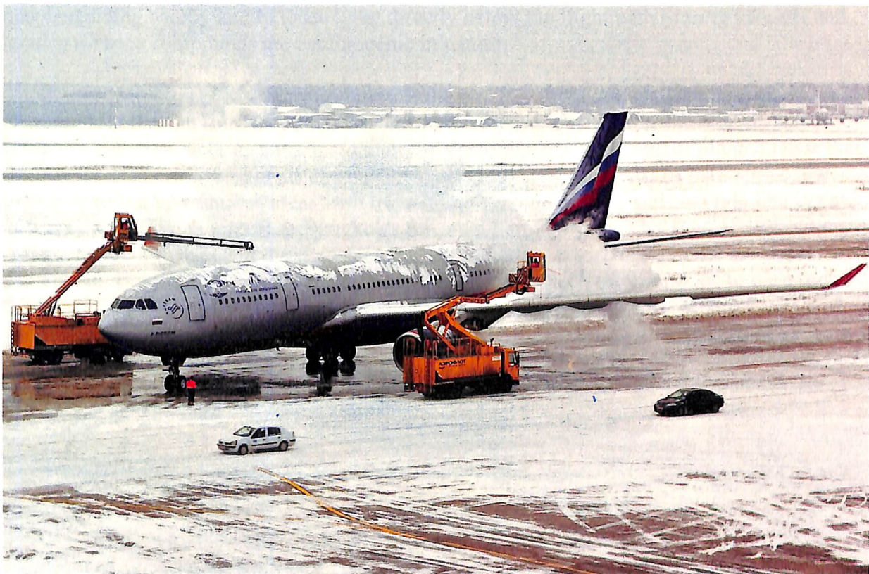
Illustration 3: De-icing of an Aircraft.
