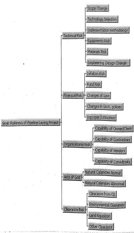
ANALYTICAL HIERARCHY PROCESS (AHP) MODEL FOR RISK DETERMINATION IN PIPELINE LAYING PROJECTS
