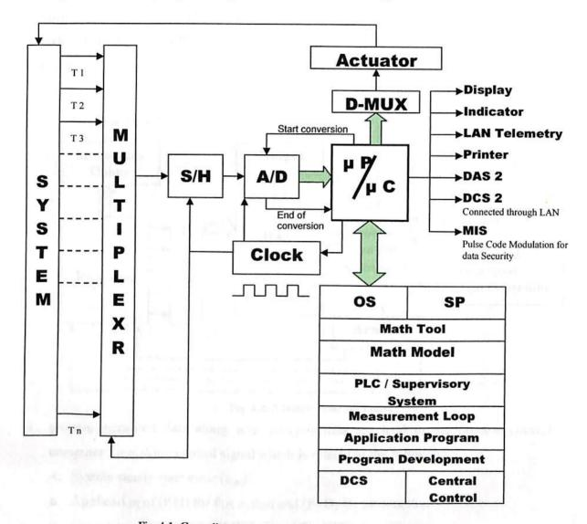
Fig. 4.1: Centralized/ Distributed Control System architecture
