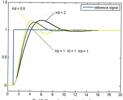
Fig. 4.7: Change of response for varying K
