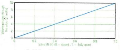
Fig. 7.2 Flow / lift curve for a linear valve
