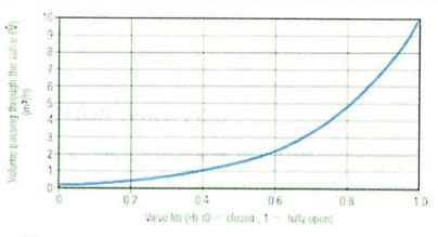
Fig. 7.3: Flowrate and valve lift for an equal percentage characteristic
