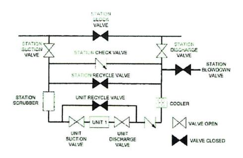
Fig. 3.1: Station Shutdown Restartable
