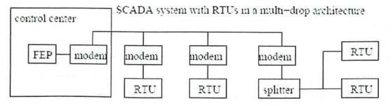
Fig.5.7: Typical SCADA system configuration
