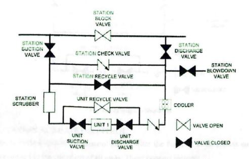
Fig. 3.2: Station Shutdown Lockout
