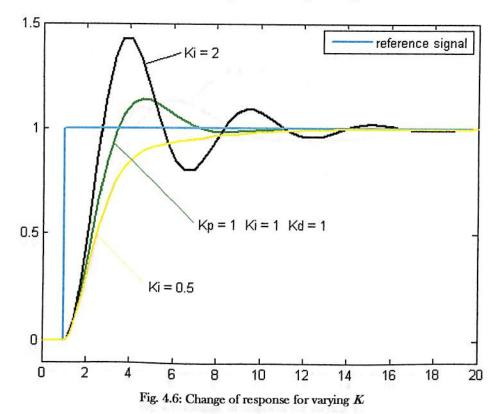
The integral term (when added to the proportional term) accelerates the movement of the process towards set point and eliminates the residual steady-state error that occurs with a proportional only controller. However, since the integral term is responding to
