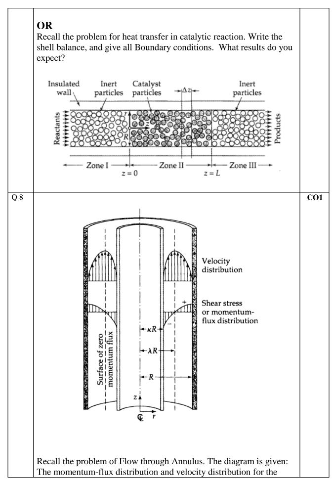
upward flow in a cylindrical annulus. Note that the momentum flux changes sign at the same value of r for which the velocity has a maximum. All the notation has its usual meaning. Derive an expression for velocity distribution, shear stress distribution, avg. velocity, maximum velocity and give full justifications.
