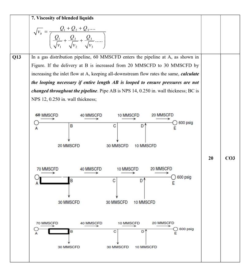
Pipe CD is NPS 10, 0.250 in. wall thickness; and DE is NPS 12, 0.250 in. wall thickness. The delivery pressure at E is fixed at 600 psig. The pipe lengths are as follow: AB = 12 miles; BC = 18 miles; CD = 20 miles; DE = 8 miles
