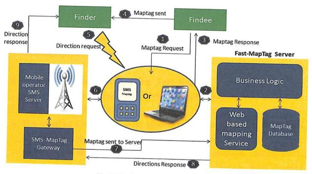
Fig.5.1 Fast map tag system flow
