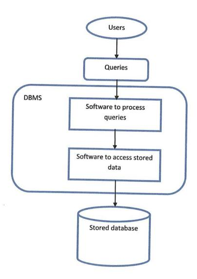
Fig. 3.5 A simplified database system environment.
