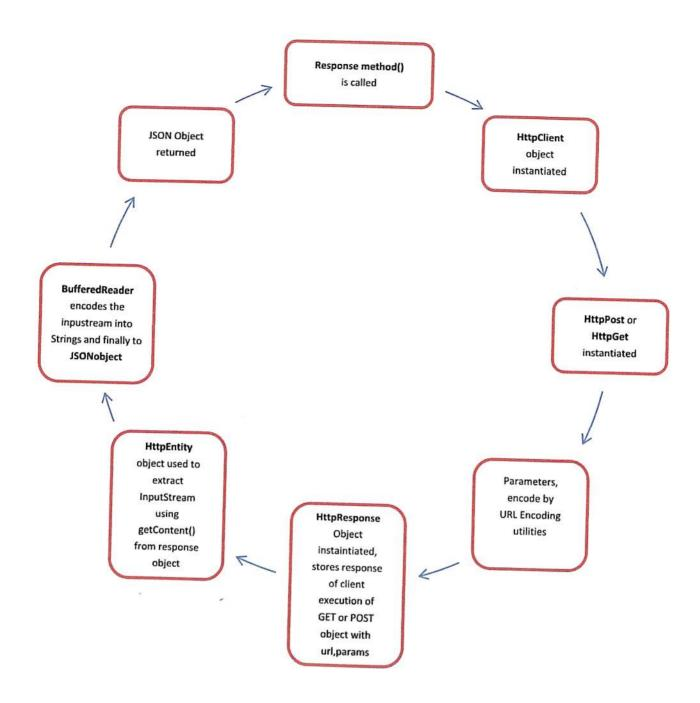
Fig6.2 Response method() execution cycle in Android
