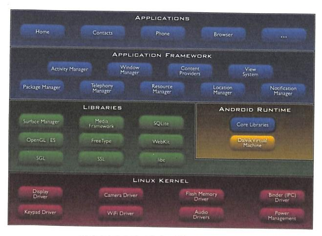
Fig. 3.1 Android Architecture [Courtesy Source: http://developer.android.com/guide/basics/what-is-android.html]
