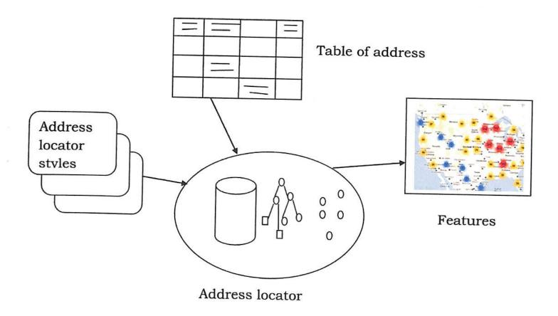
Fig. 3.4 Geocoding Process
