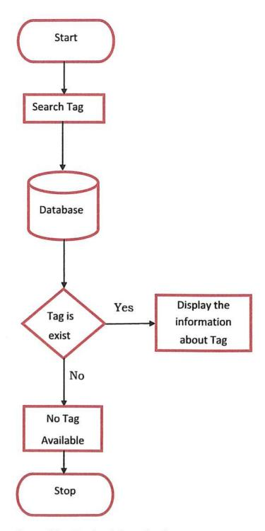
Fig 6.5 Flow chart of Tag Retrieval form database
