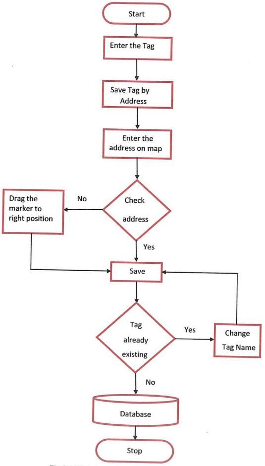
Fig 6.4 Flow chart of creating tag and save with address
