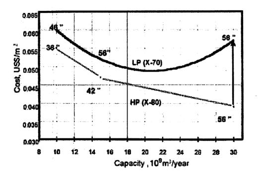
Figure 23. Long distance transportation cost for a large gas quantities, source IFP
