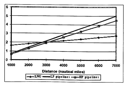
Figure 25 Pipes /LNG competition for 10\*10 $^9$  m $^3$  /year capacity, in USD / MM BTU
