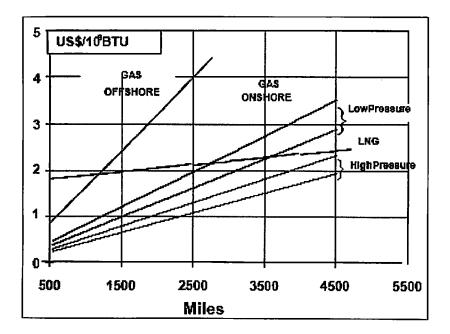
Figure 24 Pipes /LNG competition for 30  $*10^9$  m<sup>3</sup> /year capacity. Source ENI.
