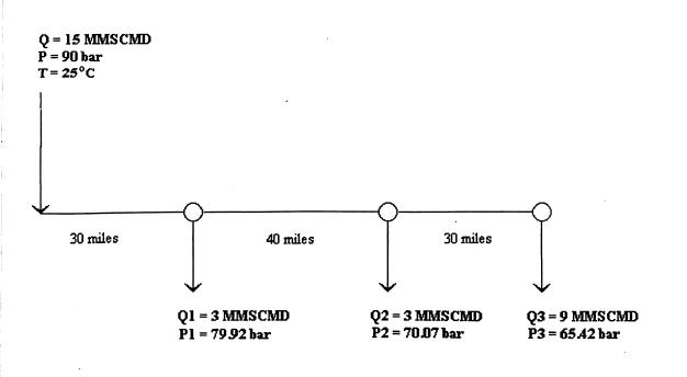
(Figure 07 – Flow diagram for case 5)
