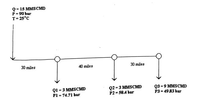
(Figure 10 – Optimized flow diagram)
