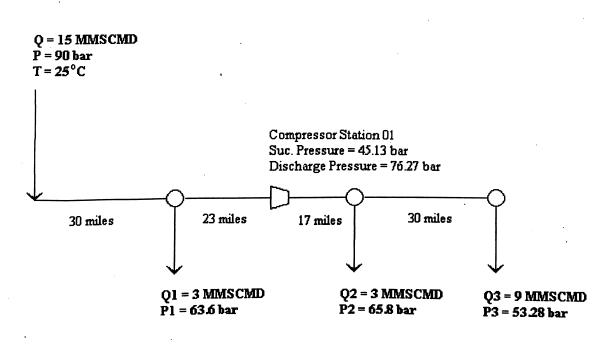
(Figure 03 – Flow diagram for case 1)
