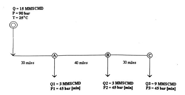
(Figure 01 -- Basic system flow diagram)
