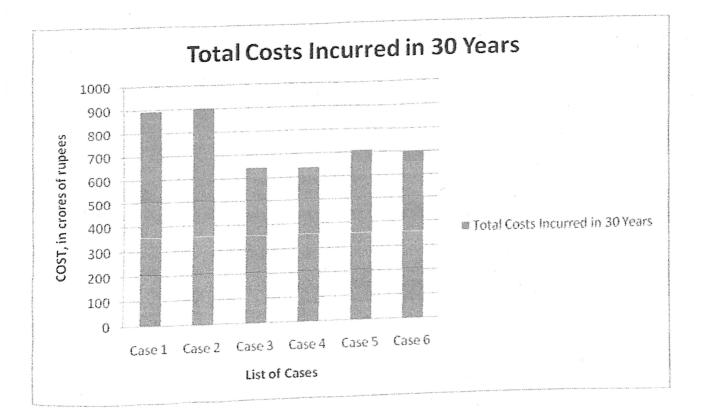
The Hydraulic analysis was performed using the Panhandle B equation. The cost analysis was conducted taking into account the various steel cost, construction cost, investment and operating costs. The results show that, case 4, i.e. the 22 inch pipe with X 70 grade proved to be most economical according to the graph.
