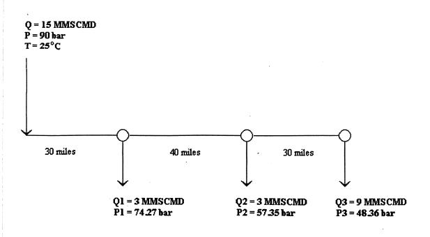
(Figure 05 – Flow diagram for case 3)
