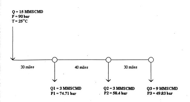
(Figure 06 – Flow diagram for case 4)
