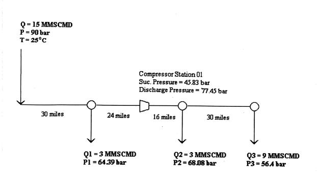
(Figure 04 – Flow diagram for case 2)
