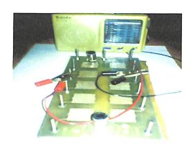
Figure 12: Photograph of small fuel cell with transistor radio
