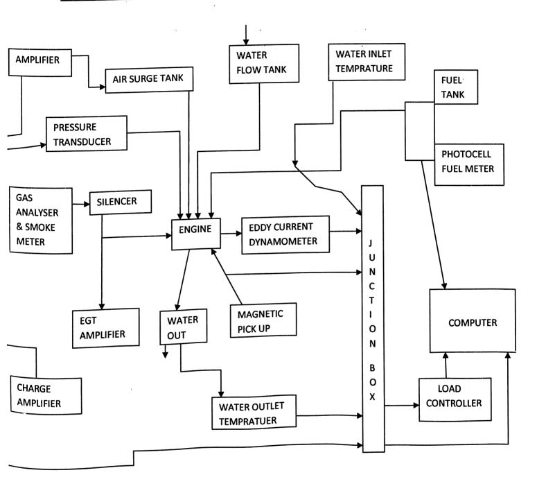
**4.1.1** <u>Engine</u>: Engine used in the experiment is a 4 stroke cycled engine made by kirloskar oil engine limited. in a water cooled, naturally aspirated, direct injection engine having specifications:-
