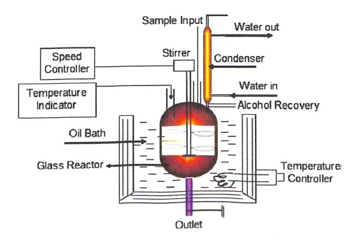
Bio-diesel is formed from oils by a process called 'TRANSESTERIFICATION' in which vegetable oil is reacted with an alcohol in the presence of catalyst and glycerol is formed as a by product. Basically we take 1000ml of jatropha oil which is reacted with methyl alcohol(200 ml)
