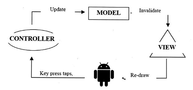
Figure 5.4. Model-view-controller concept
