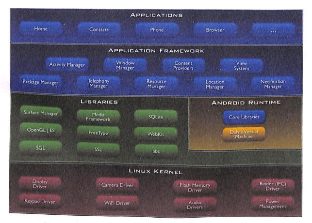
Figure 3.1 Android Architecture [( Source, courtesy http://developer.android.com/guide/basics/what-isandroid.html)]
