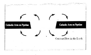
FIGURE NO.2 Cell Caused by Different Environments
