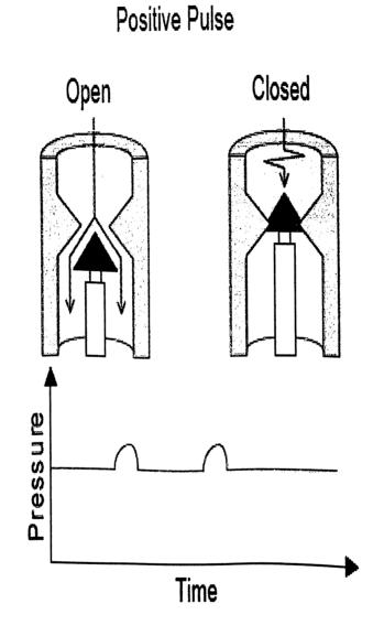
Figure 4-35 Positive pulse telemetry
