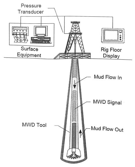
Figure 4-33 Mud pulse telemetry
