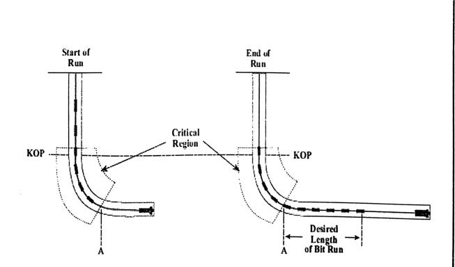
The length of heavyweight must be increased so that heavyweight drillpipe is at point A at the beginning of the run, as well as the end. At the end of this run, compressive forces at point A may have increased to the critical buckling force, and drillpipe will buckle. Therefore, heavyweight drillpipe should be used here.
