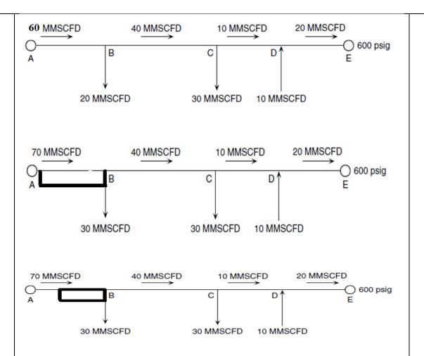
Pipe CD is NPS 10, 0.250 in. wall thickness; and DE is NPS 12, 0.250 in. wall thickness. The delivery pressure at E is fixed at 600 psig. The pipe lengths are as follow: AB = 12 miles; BC = 18 miles; CD = 20 miles; DE = 8 miles
