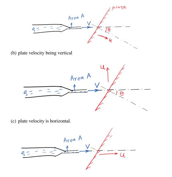
The inlet water velocity corresponding to the hydropower plant is 100 m/s and the blade (flat plate, in our case) velocity at the centerline is 60 m/s. Answer these:
