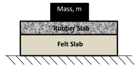
Q.6 The amplitude of the system shown decreases to 25 % of the initial value after 5 consecutive cycles. Determine damping coefficient c of the system if k 40 N/cm and the mass m=4 kg. [15 marks]
