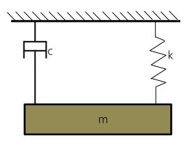
Q.7 A body of mass 5 kg is supported on a spring of stiffness 2000 N/m and a dashpot. The dashpot produces a resistance of 2 N at a speed of 1 m/s. in what ratio amplitude of vibrations will be reduced after 4 cycles? [15 marks]
