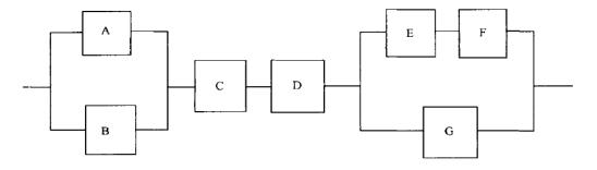
b) Assume that the time to failure for each component has an exponential distribution. The failure rates are as follows:  $\Lambda_A = 0.0005/\text{hour}$ ,  $\Lambda_B = 0.0005/\text{hour}$ ,  $\Lambda_C = 0.0003/\text{h}$ ,  $\Lambda_D = 0.0008/\text{hour}$ ,  $\Lambda_E = 0.0004/\text{hour}$ ,  $\Lambda_F = 0.006/\text{hour}$  and  $\Lambda_G = 0.0064/\text{hour}$ . Find the
