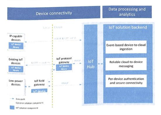
Figure 11: IOT Solution Architecture
