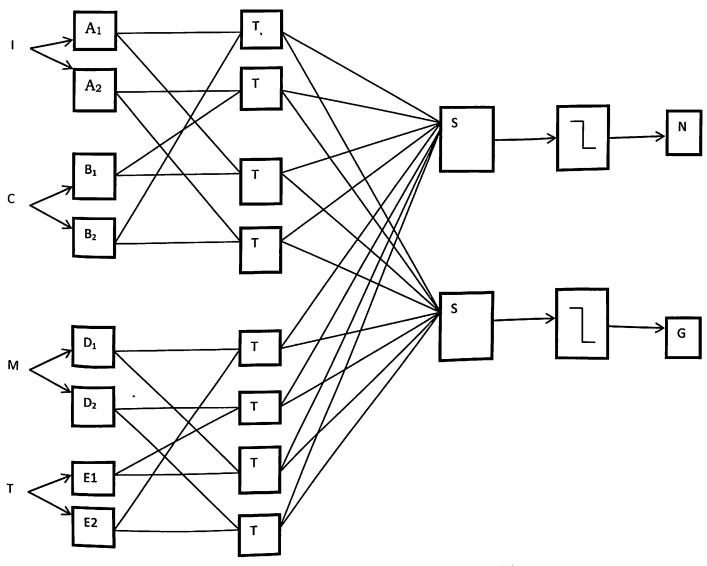
Figure 5.1: Flow of Hybrid Neuro Fuzzy Model
