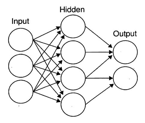
Figure 1.5: Three layer perceptron
