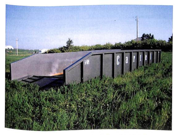
Figure 4.3: Example of a Three Sided Shale Bin
