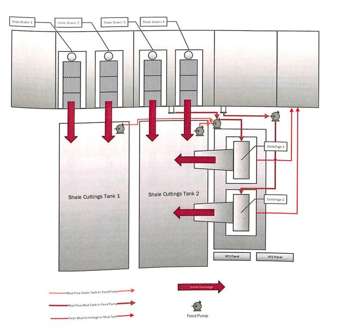
Figure 4.1: Centrifuges set up in parallel
