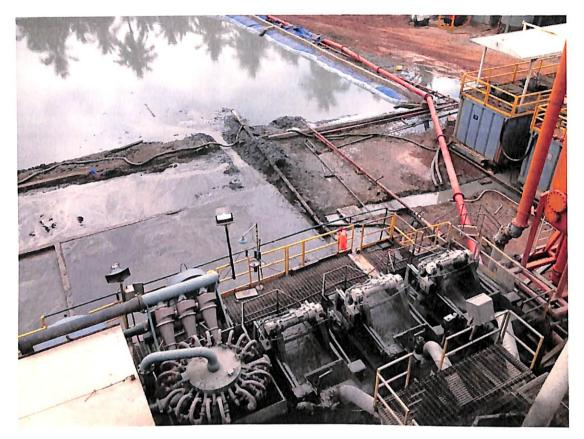
Figure 1.2: Overflow into water sump
