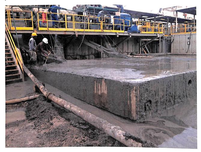
Figure 1.1: Waste pit overflowing
