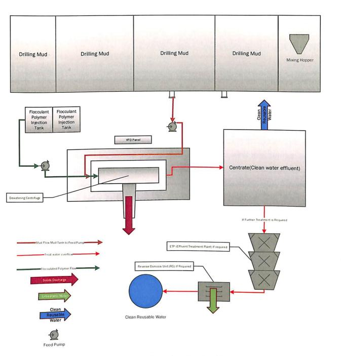
Figure 4.4: Dewatering Configuration Detail and Recycling Setup
