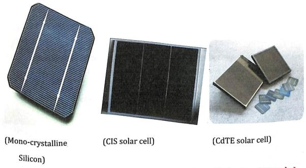
Fig 1.3 DIFFERENT TYPES OF SOLAR CELLS (Ref: solarstere.co.kr)
