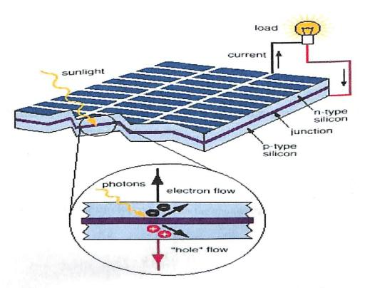
Fig 2.1: SCHEMATIC DIAGRAM OF SILICON SOLAR CELL (Ref: www.solarpower2day.net)
