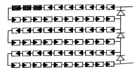
Fig 2.14 PARTIALLY SHADED MODULE (Ref: www.sciencedirect.net)
