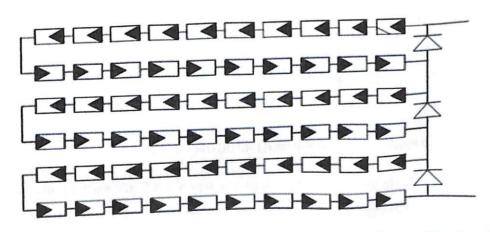
Fig 2.13 MODULES WITH BYPASS DIODES (Ref: www.sciencedirect.net)
