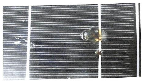
Fig 2.12 SOLAR MODULE WITH HOTSPOT (Ref: www.sciencedirect.net)
