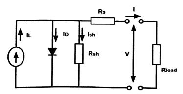
Fig 2.2 SINGLE DIODE MODULE PV CELL (Ref: www.sciencedirect.net)
