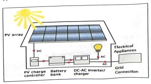
Fig 2.17 SOLAR PV BATTERY CONNECTED SYSTEM (Ref: solarshop.co.uk)
