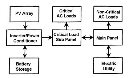
Fig 2.18 SOLAR PV BATTERY CIRCUIT DIAGRAM (Ref: www.fsec.ucf.edu)
