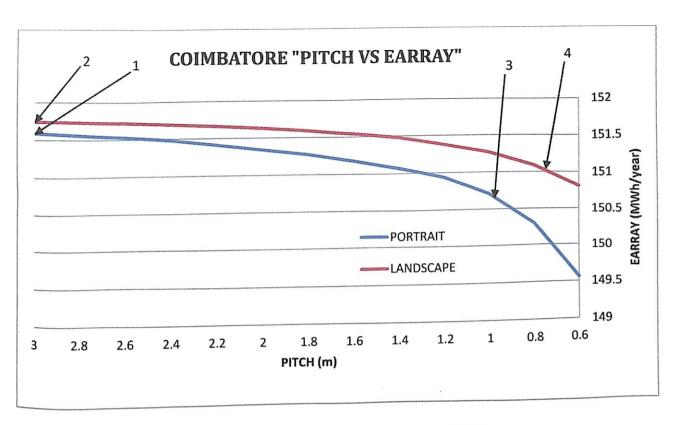
Fig 3.22 PITCH VS EARRAY FOR COIMBATORE
