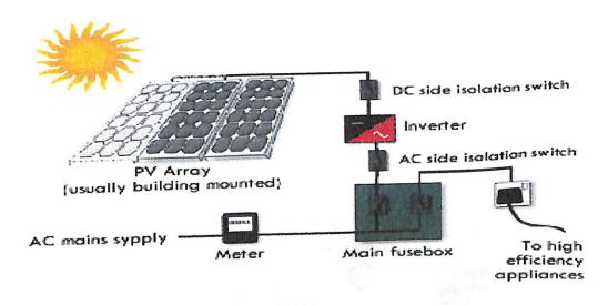
Fig 2.15 SOLAR PV GRID CONNECTED SYSTEM (Ref:solarshop.co.uk)
