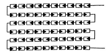
Fig 2.11 MODULE WITHOUT BYPASS DIODE (Ref: www.sciencedirect.net)
