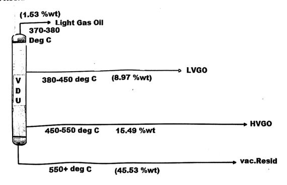
Figure 8:- Schematic diagram of VDU with different cut.
