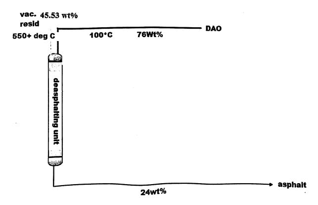
Figure 9- Schematic scheme of Solvent Deasphalting Unit with material balance
