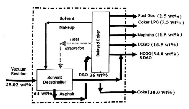
Figure 18: - Schematic diagram of integrated solvent Deasphalting and Delayed coking unit
