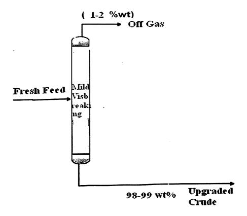
Figure 15: - Mild Visbreaking Unit
