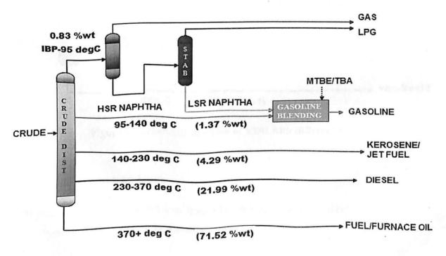
Figure 7: - Schematic diagram of CDU with various cut
