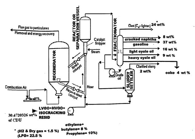
Figure 20: - Material balance of feed and product in FCCU [17].
