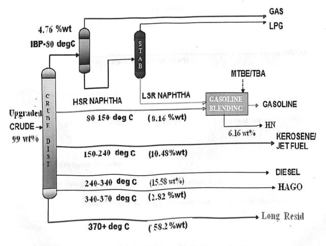
Figure 17: - Schematic Diagram of Crude Distillation unit with various cuts
