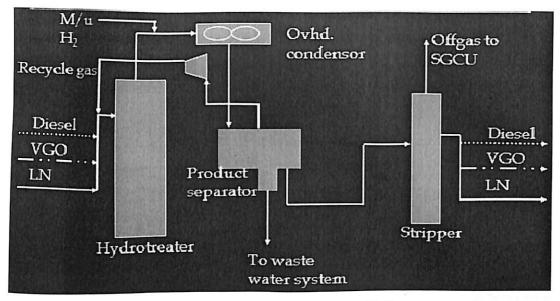
Figure 21: - Schematic diagram of Hydrotreater unit
