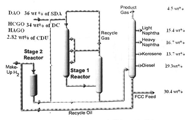
Figure 19: - Schematic diagram of TSR Isocracking Unit
