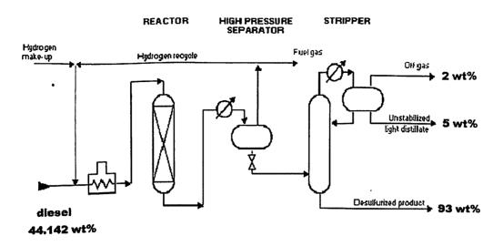
Figure-12-Diesel Hydrodesulfurization Unit
