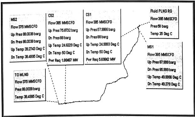
Figure 4: Model obtained at 375 MMSCFD
