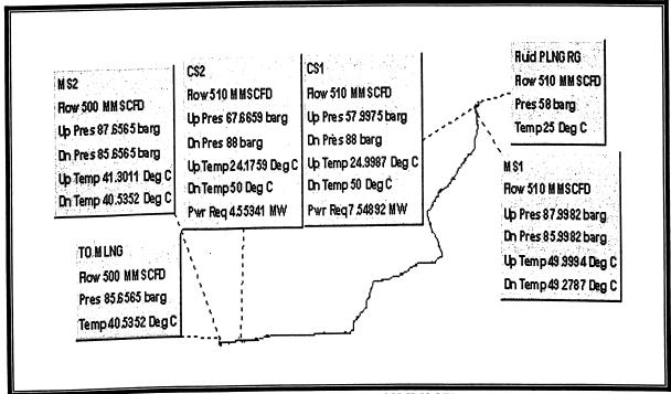
Figure 6: Model Obtained at 500MMSCFD
