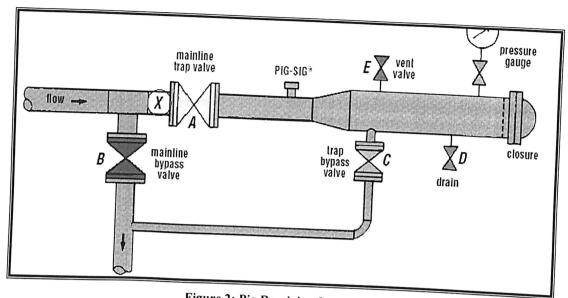
Figure 2: Pig Receiving System
