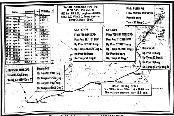
Figure 7: Model as per client at 750MMSCFD
