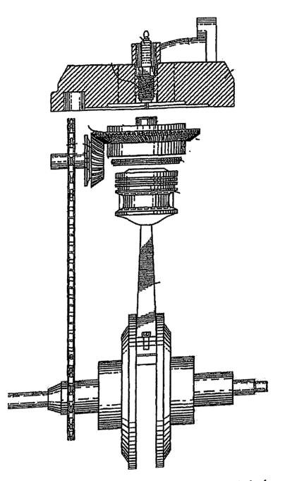
Figure 2. Front view of the Disc Valve System without the cylinder box and cylinder.
