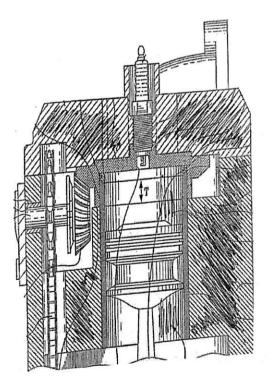
Figure 4. Sectional view of the Disc Valve System
