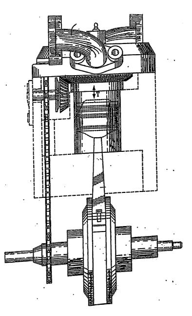
Figure 1.Front view of the Disc Valve System showing the cylinder box and cylinder in
