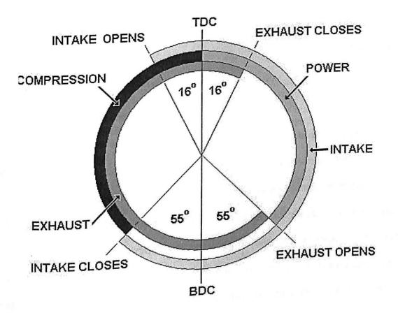
Figure 1. Valve timing diagrsm
