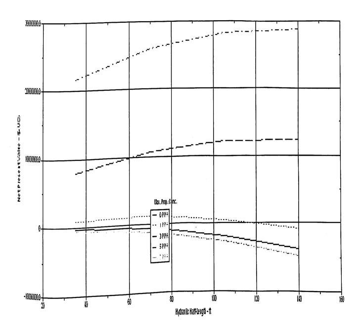
Figure 9. Plot of  $x_f vs NPV$
