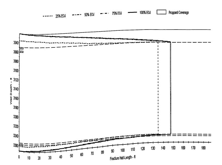
Figure 13. Fracture growth with well depth
