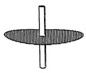
Figure 2. A Horizontal Fracture Geometry
