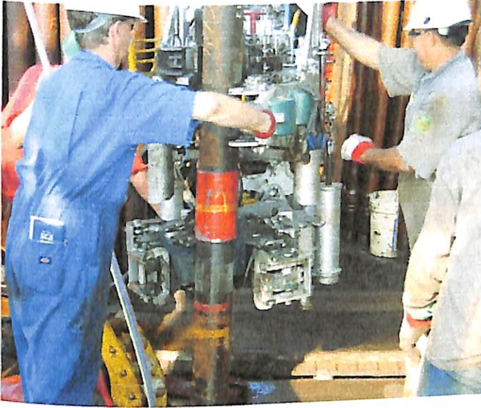
Figure 2.20 Preparing to make-up chrome tubing
