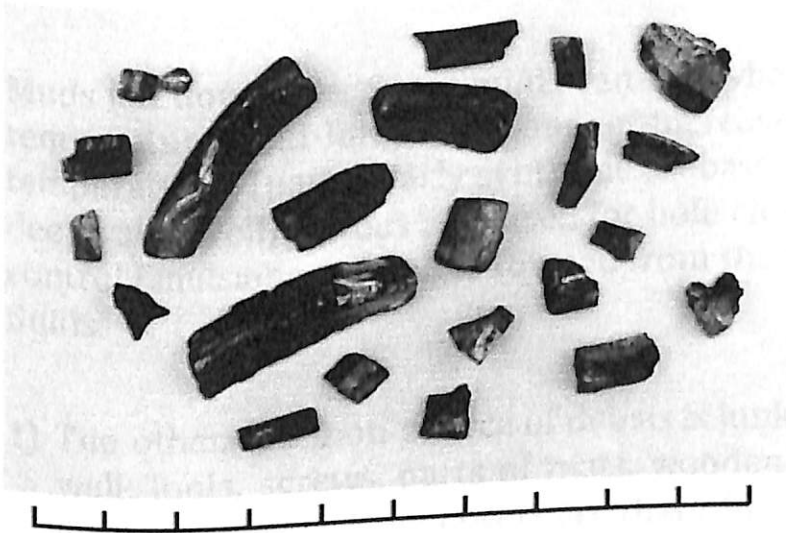
Figure 2.3 Debris from the milling of a packer.
