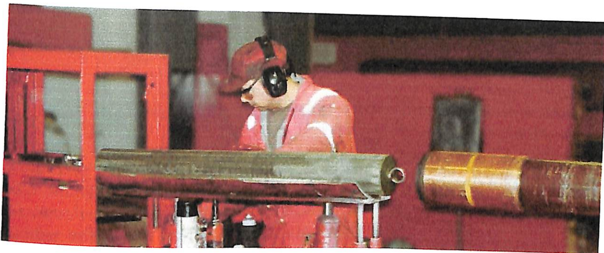
Figure 2.16 Drifting tubing before shipment to the wellsite.
