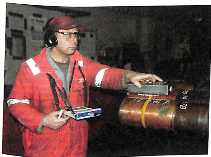
Figure 2.17 Measuring pipe by laser before shipment to the wellsite.
