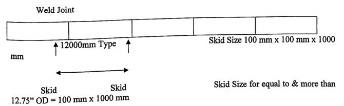
Maximum offset of the same nominal wall thickness pipe shall not be more than 1.6 mm. Maximum length of weld string shall be 1000 Meters. And the off-set may be checked by using dial gauge.
