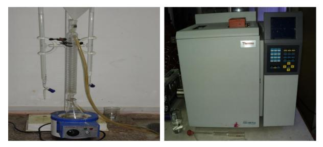
Fig. IV.6 Set-up for COD with heating mantle
