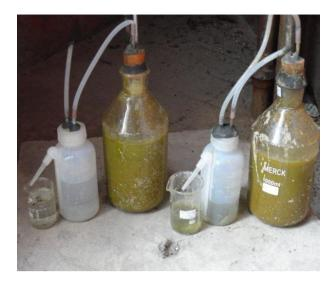
Fig. IV.8 Laboratory scale digesters
