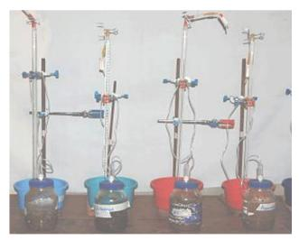
Fig. 4.2 Batch stirred tank reactor with water displacement
