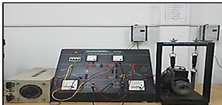
Fig.5.9: Experimental set up for new design 1 H.P Motor [169]
