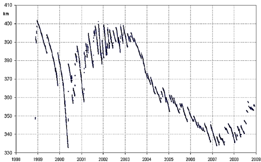
Figure (4.10) Orbit Decay of the International Space Station (ISS) [96]
