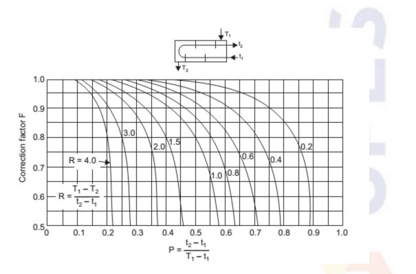
Correction factor F for shell-and-tube heat exchangers with one shell pass and any multiple of two tube passes (2, 4, 6, etc., tube passes).
