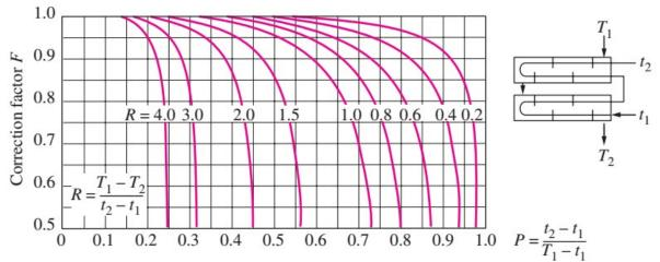
Two-shell passes and 4, 8, 12, etc. (any multiple of 4), tube passes
