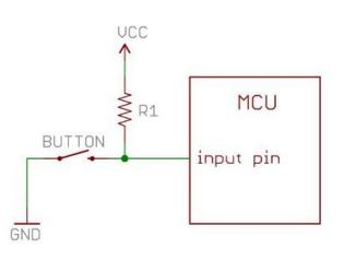
When the button is open what will be the input voltage to the microcontroller? Define it with reference to pull up and pull down concept.
